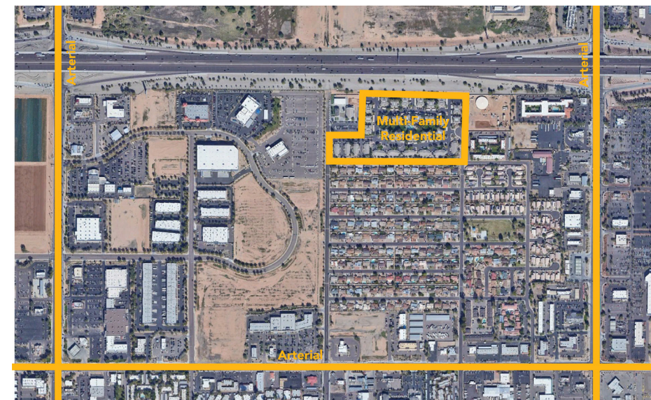
Figure 9.10 Example of a development that does not meet Standard 24 . There is no direct access onto an arterial roadway. If access had been provided to the arterial roadway through one of the commercial centers, it would comply with Standard 24. Since access is through a single-family residential development, it does not conform to Standard 24. Location: North Subdivisions, Goodyear, Arizona
